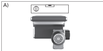
A) Level the conveyor
